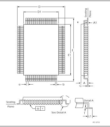
Figure 27. Dimension Diagram for the 82555 QFP
